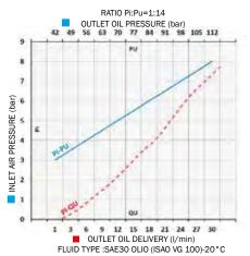
These pumps are advised for the transfer of low-high viscosity oil and similar fluids for medium-long distances. The delivery capacity of a pump varies according to particular applications and combinations. The operating pressure may vary between a minimum of 3 bar and a maximum of 8 bar.
